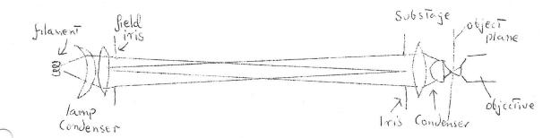
The lamp condensing lens images the filament of the lamp on to the substage condenser back lens and the substage condenser images the field iris on to the specimen.
